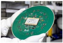
and enables troubleshooting of particles down to 0.1  $\mu m$  in gas and vacuum lines in any areas of the fab 24/7.
